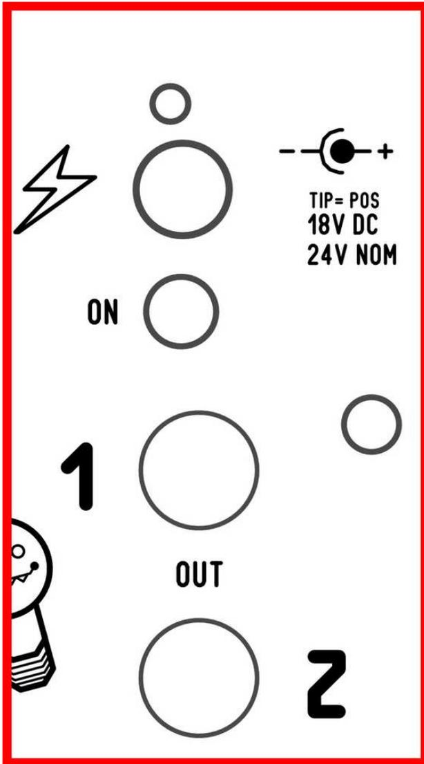
The Dwarf Star synthesizer is using a DC to DC converter. The requirement needed for the converter to do it's magic is to input a 18v to 24v DC adapter rated at minimum 3A. 2 Amps might work, but I supply and use 3 amps. I like to supply more current then needed. The total amperage is shared by the rails. So the synyth might use 1.5A for +12v and 1.5A -12v.
