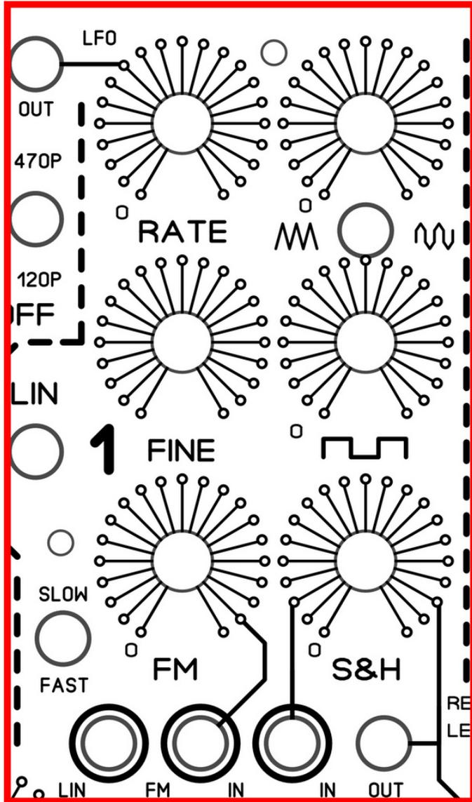
This lfo is using a triangle core design also. But this design is not a discrete transistor based core like the vco's. It is using an OTA LM13700 chip to form the triangle wave. I decided on this particular design because it uses a very unique Linear voltage control. This Linear control does not act the same when implemented on the VCO's for example. The linear control can sound Arpeggio like and very musical.
