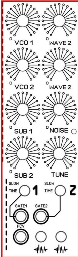
The VCO1 knob and wave 2 knob are considered a set. VCO2 and wave 2 knobs right below them are also a set.
