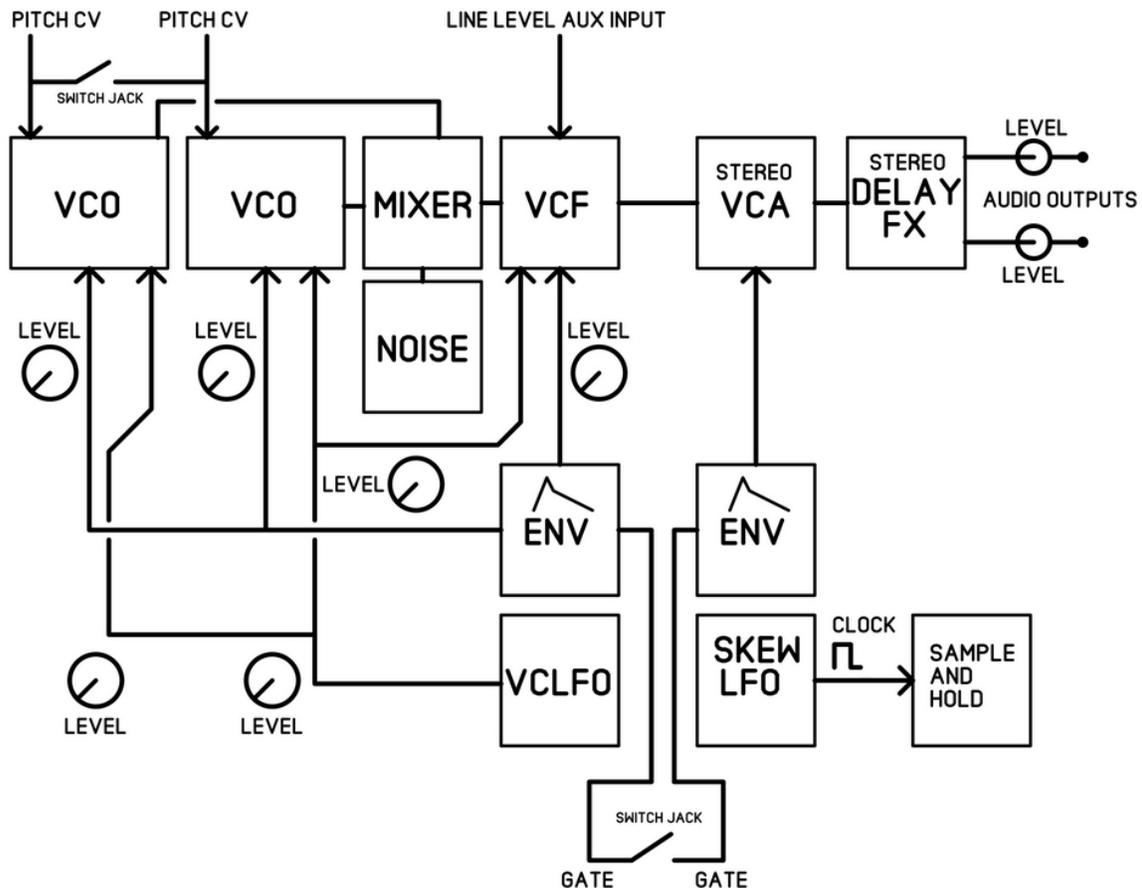
The synthesizer has some basic internal patching. The first envelope generator and vc-lfo are internally patched to the VCO's, and the VCF. I installed a dedicated 'Level' knob for each internal patch. Each level knob has either an on/off toggle switch or an invert switch.
