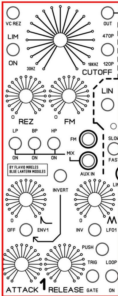
The Dwarf Star Synthesizer does not have a 'cascaded transistor' filter or Moog vcf. You have too much of those in your studio already. This design uses a cool audio v2164 quad vca to do low pass, band pass, and high pass. I internally connected those outputs to toggle switches, and then those internally mix into a hidden mixer section inside. Each filter flavor was internally amplified for proper levels. So no matter which toggle switch you use, the output will be seamless and mix nicely.
