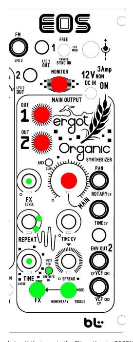
On power up there is an internal circuit that resets the FX section to GREEN, meaning FX ON.
