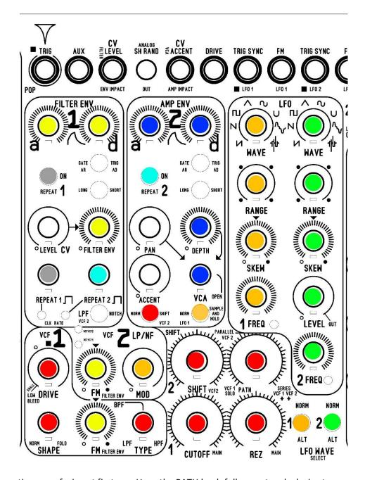
The filter section a confusing at first use. Have the PATH knob fully counter clockwise to use as a normal solo filter. SHIFT knob is basically Cutoff knob for Filter #2. You only use SHIFT knob if Path knob is set up clockwise into PARALLEL MODE and SERIES MODE.
