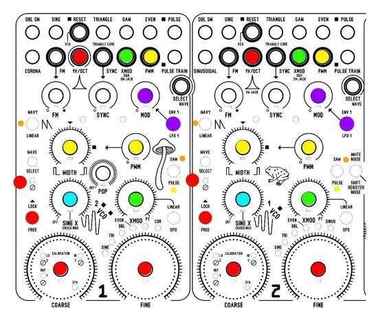
Red Section: pitch tuning related controls. Coarse knob, Fine Tune knob, Lock Switch, and Trimmers.
