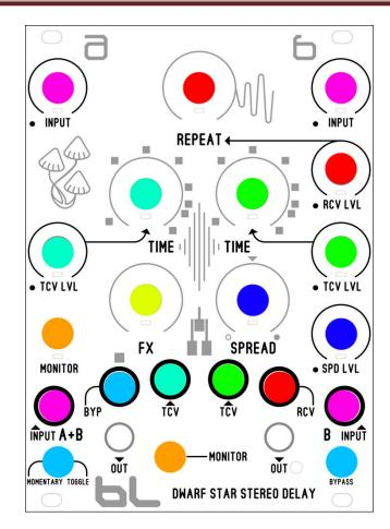
Pink Knob and Input Jacks: use these to patch an audio source into the module. The input knobs are used to adjust the input level. If you hear distortion, simply lower the level knobs. You can patch a mono signal input the left INPUT A+B jack and it will internally patch to the other B input jack using the switch jack.
