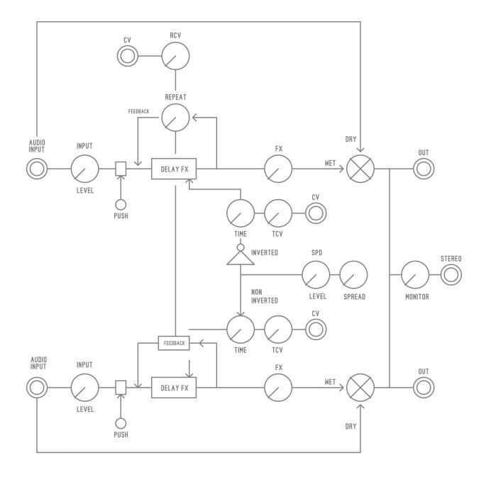
BLM Dwarf Star Stereo Delay MK2 Width: 18hp Single Level PCB, Skiff compatible. BLM Standard Ribbon Cable: 10 pin to 16 pin Current: +81mA,-38mA Outputs: 1K Ohm, -5v/+5 Time CV: 68K Ohm, -5v/+5 Repeat CV: 100k Ohm, -5v/+5 Inputs: Expect -5v/+5 signals Middle 5 Potentiometers are D Shaft Side Potentiometers are Knurled Shaft
