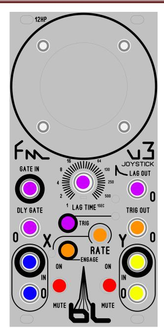
Dark Blue Jacks: input and output for the x-axis portion of the joystick. This is a bi-polar positive and negative circuit. When nothing is patched into the input jack, roughly -5V/+5v is used for the output.
