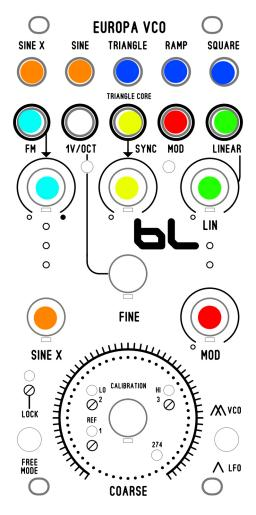
Orange: Sine, and Sine X. These are sine wave outputs. The internal sine wave was buffered twice so that two outputs were possible. One output is direct out, and the SINE X has output level control. The SINE X is a good way to crossmod patch another Europa VCO. Both SINEX and SINE outputs can be used simultaneous.
