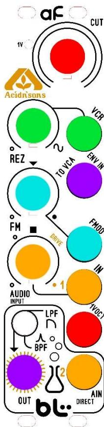
**Red Section:** Cutoff Knob and 1V Octave input jack. This section controls the frequency cutoff for the filter. Use the 1v Octave input jack for Self-Oscillation Scale tracking.
