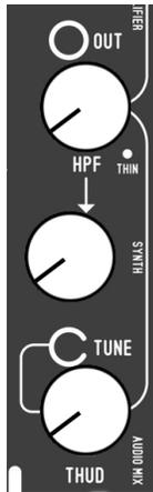
The THUD oscillator sometimes it can be too much mid range. The HPF (High Pass Filter) above the THUD tuner is used to cut off some of the low frequencies.
