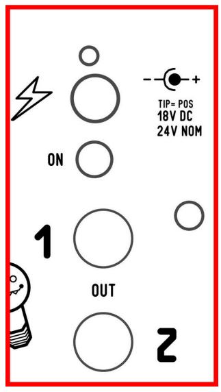
The Dwarf Star synthesizer is using a DC to DC converter. The requirement needed for the converter to do it's magic is to input a 18v to 24v DC adapter rated at minimum 3A. 2 Amps might work, but I supply and use 3 amps. I like to supply more current then needed. The total amperage is shared by the rails. So the synth might use 1.5A for +12v and 1.5A -12v.
