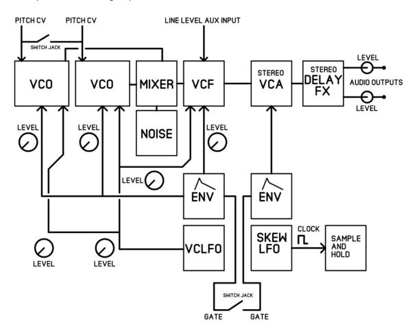
The synthesizer has some basic internal patching. The first envelope generator and vc-lfo are internally patched to the VCO's, and the VCF. I installed a dedicated 'Level' knob for each internal patch. Each level knob has either an on/off toggle switch or an invert switch.
