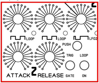
Each envelope generator is capable of internally looping and cycling. Each generator also has it's own independent Loop rate control. In this particular diagram, middle loop knob is for envelope #2. You turn on the loop feature with the toggle switch.
