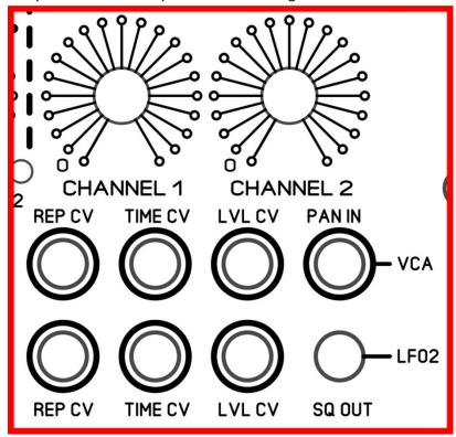
The top row of CV inputs for the Delay section is internally switch jack connected to the bottom row CV inputs. I did this so that you could control both delays with minimal patching. If your require independent cv control simply plug it in, it will break the switch jack connection.
