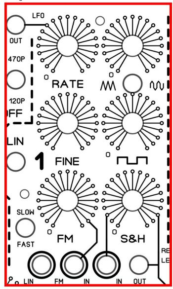
This Ifo is using a triangle core design also. But this design is not a discrete transistor based core like the vco's. It is using an OTA LM13700 chip to form the triangle wave. I decided on this particular design because it uses a very unique Linear voltage control. This Linear control does not act the same when implemented on the VCO's for example. The linear control can sound Arpeggio like and very musical.
