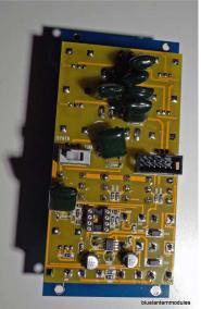
On the back of the unit there is a slide switch. That is used to select how the front Direct Input will act. You can either select it for synth level signals or line level signals. What it does exactly is toggle between a 200k resistor (synth level) and a 10k resistor (for line level input). If you select the line level mode and plug in a synth level signal it will distort. You will not damage the module, it is just changing the x amplification ratio on the op-amp and therefore distorting.
